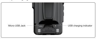
Use the matching desktop charger to charge the battery/battery-equipped transceiver. Make sure that the battery is in contact with the charger contact. When the charging indicator light is red, charging starts, and when the green light is on, charging is complete.
