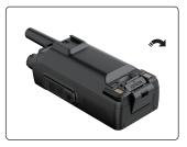
Match the top of the battery pack with the corresponding proves on the radio. Push the battery onto the bottom of the radio, buckle the safety lock. To remove the battery pack, life the safety lock and pull the battery pack away from the radio.
